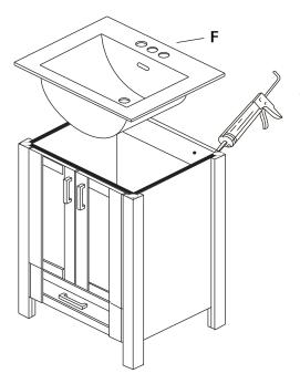
Add a small bead of silicone to the top perimeter of the cabinet where contact will be made with the sink. Then carefully place the sink on top, and immediately wipe away any visible silicone residue. Silicone is not included.
