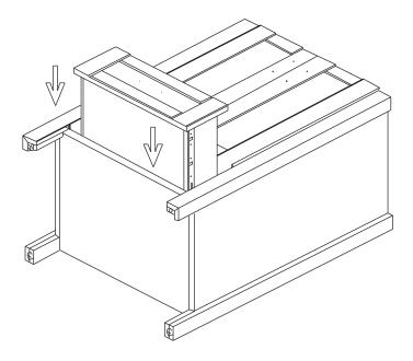
• Install all 4 leveling screws (BB) into the bottom of the legs
