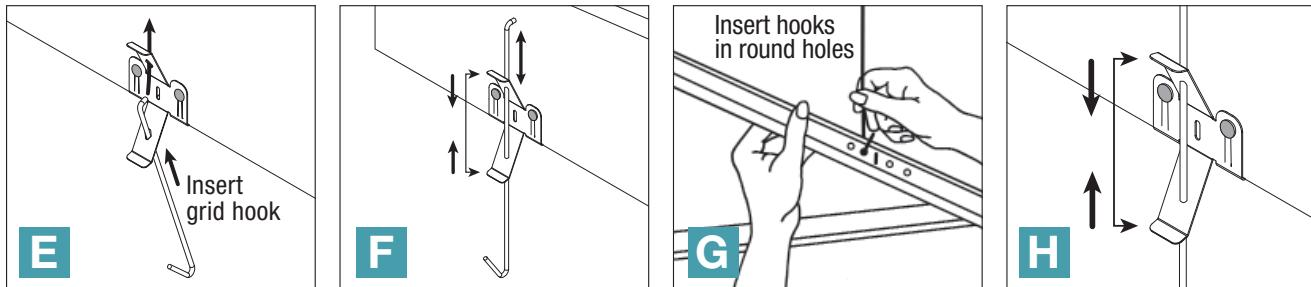
**STEP 6:** Turn all hooks in the same direction, parallel to joists. Set all hooks to about the same height.
